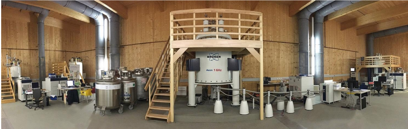
Bruker Aeon 1 GHz magnet Installed at the University of Bayreuth B_0 = 23.5 Tesla P/P_0 = 2
